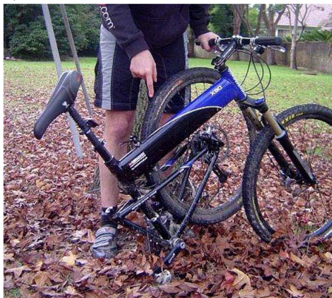
Step 3: Twist the rear triangle around
