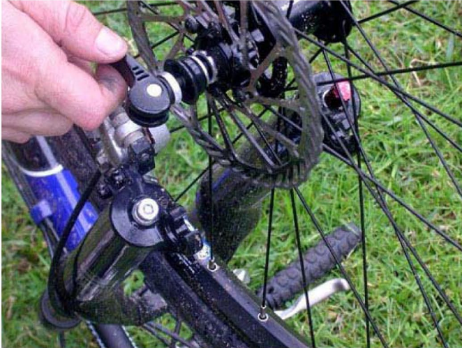
Step 4: Detail - removing the front wheel - once handed with the sprung skewer
